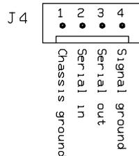
Serial cables can be ordered from Microstar Laboratories. The MSCBL 010-01 is a printer-compatible serial cable and the MSCBL 013-01 is a PC-compatible serial cable. Voltage levels on the serial connector conform to the RS-232 standard.
