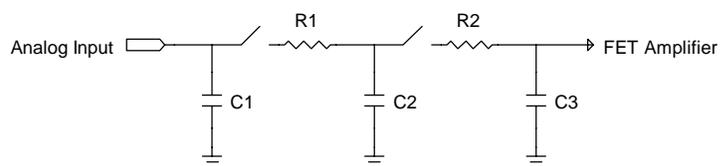
The DAP 800 and DAP 801 have fault-protected multiplexers. The following table shows typical resistance and capacitance values, in Ohms and picofarads, for fault-protected multiplexers.
