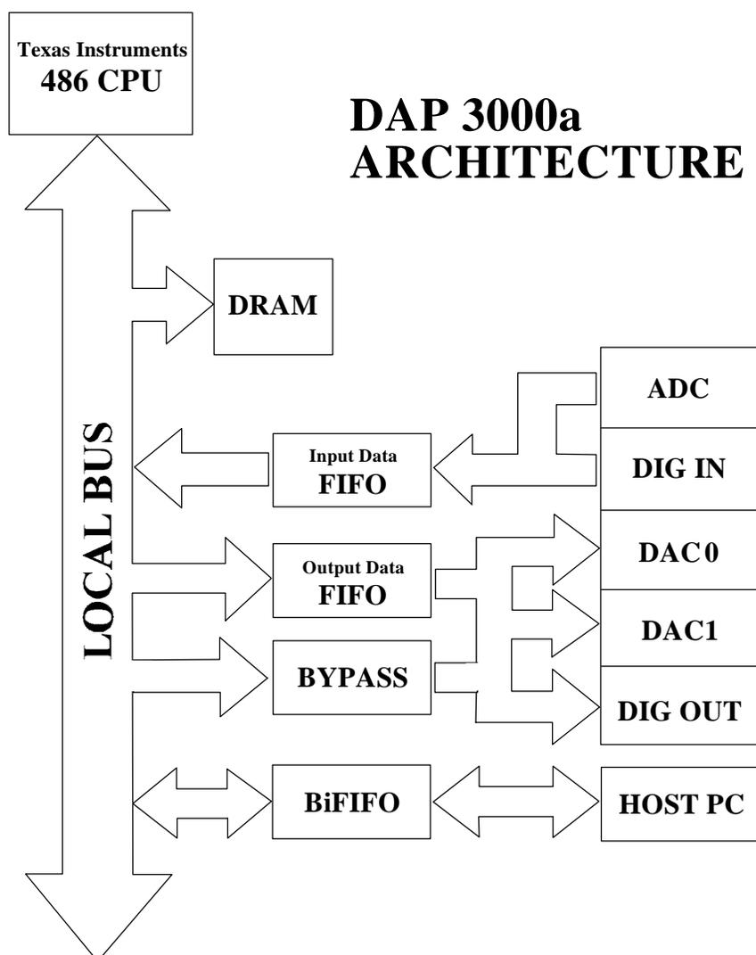
**Figure 1: DAP 3000a Data Acquisition Hardware**
