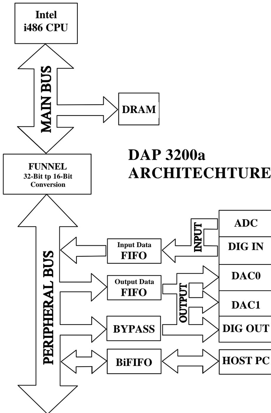
**Figure 1: DAP 3200a Data Acquisition Hardware**
