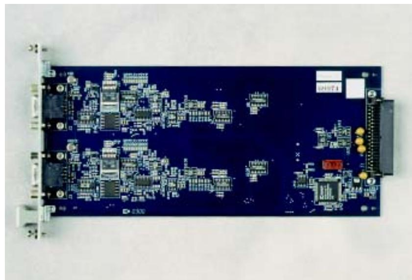
*Key Component: 2-channel MSXB 044 board with 15-pin DB connectors shown at left*
