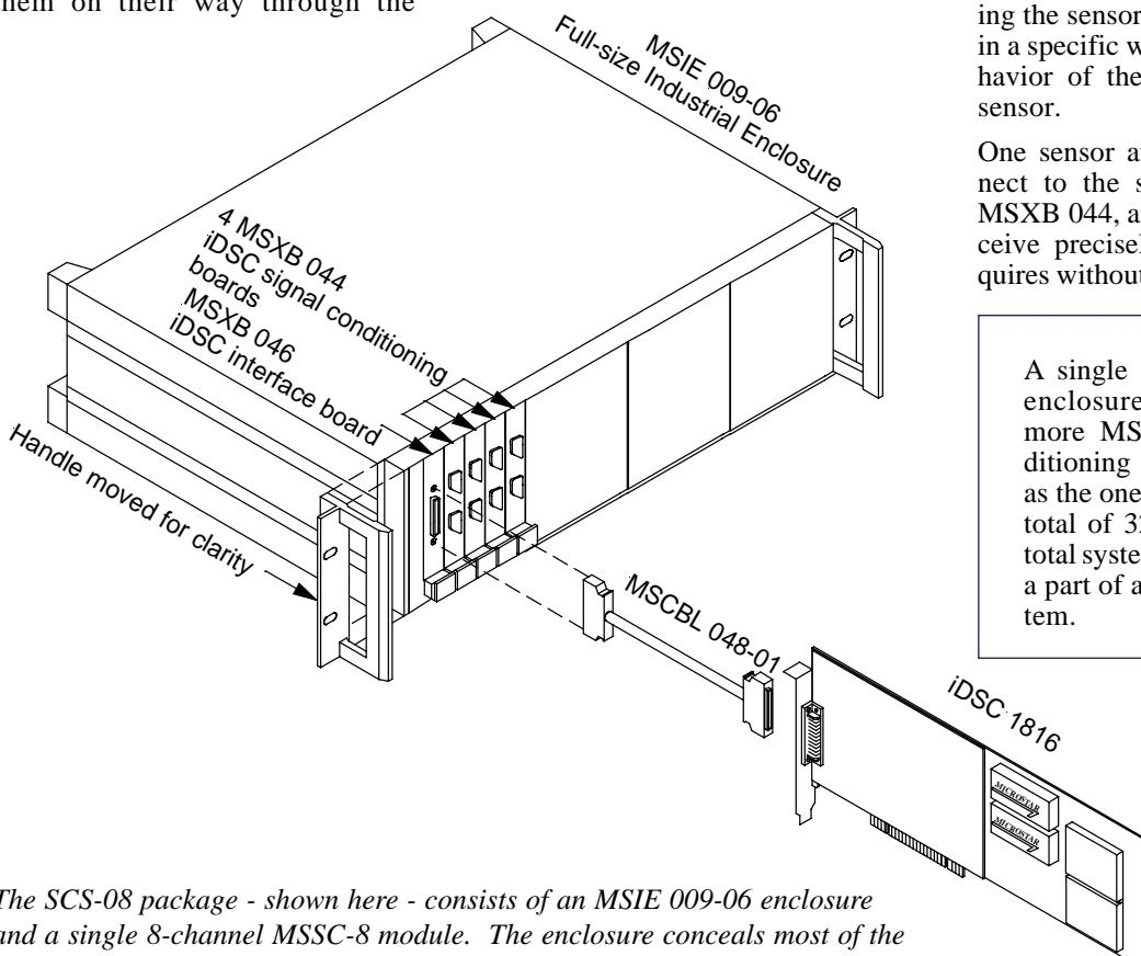
A single 19-inch industrial enclosure can hold three more MSSC-8 signal-conditioning modules, as well as the one shown here, for a total of 32 channels – as a total system on its own, or as a part of an even larger system.
