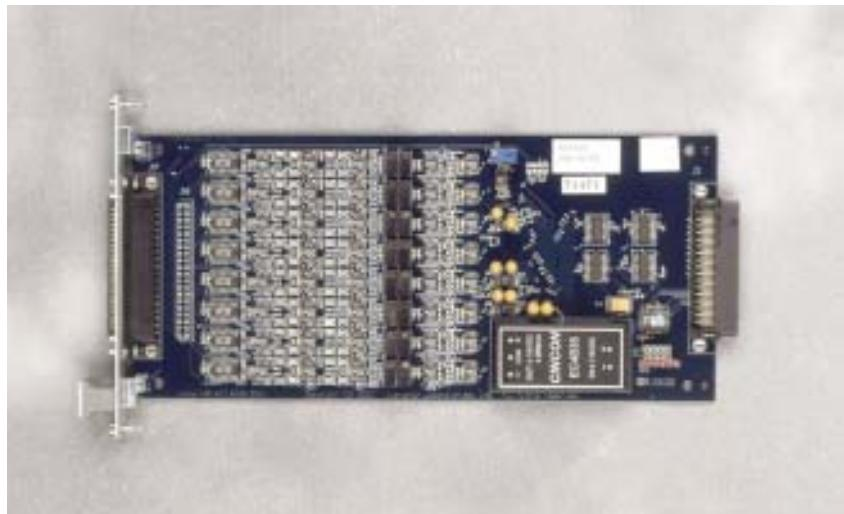
*Onboard analog filters – similar to the analog filters on the iDSC 1816 – block unwanted high frequencies on each channel of the MSXB 048, shown here.*
