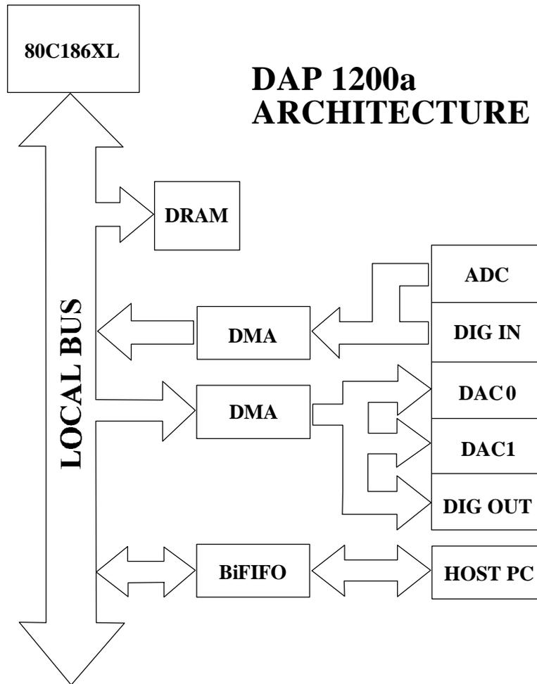
**Figure 1: DAP 1200a Data Acquisition Hardware**
