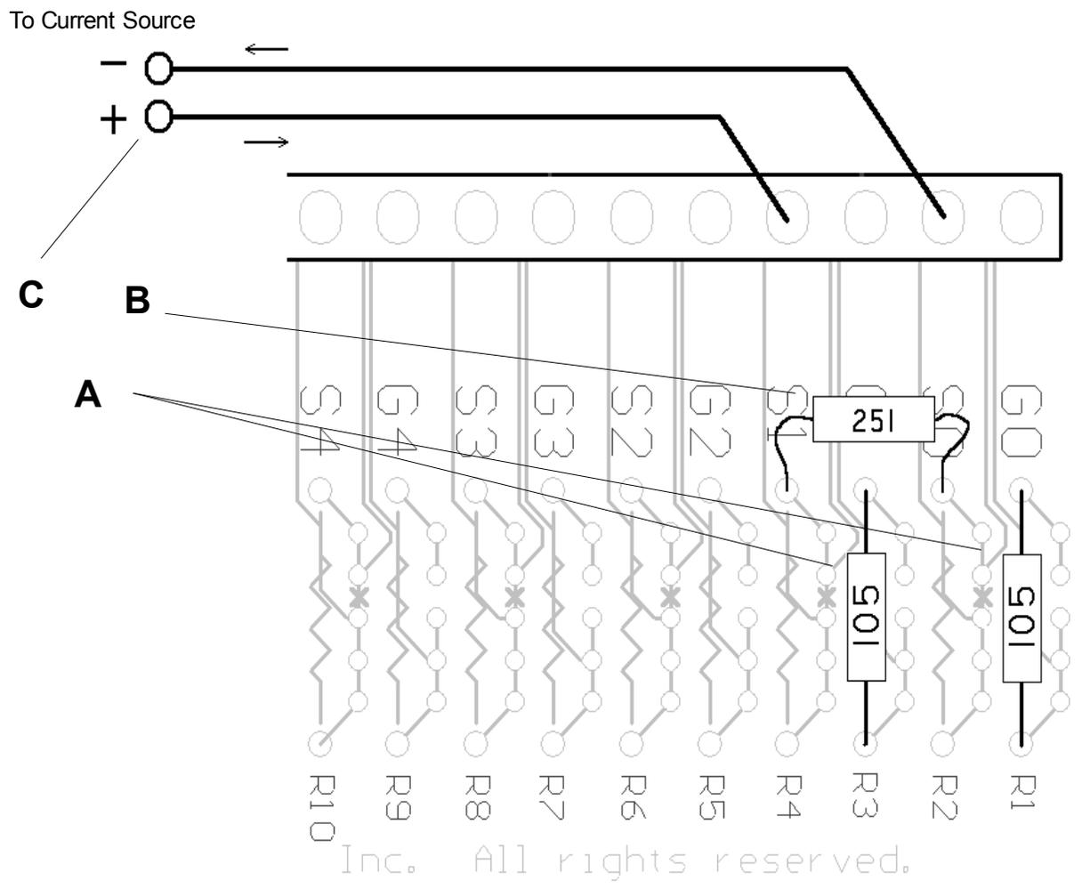
Figure 1: Connections for Differential Current Sense Measurements
